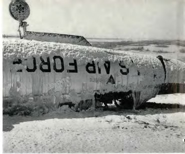
Above and right. This F-104 was using a barrier for its arrestment. Only one of the main gears caught the arresting cable and it flipped over. The pilot had no canopy, so he crawled out without trouble.
