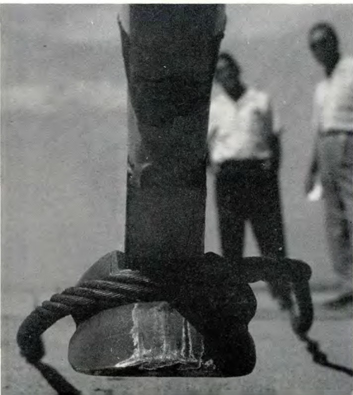
Right, solid Navy-type shoe with stellite foot plate inserted to stop excessive wear when hook is snubbed against runway to prevent skipping over cable. Below, smooth shoe will not cut or kink cable.
