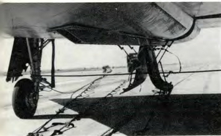
Above. To catch the arresting cable before it falls to the runway because of the excessive distance between the nosewheel and the mains, this finger slot is added to the '106 to insure engagement when using barrier. Below, many protrusions invite damage by cable.
