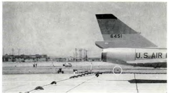
Above. The F-106 makes a perfect catch and yielding elements begin to fly. Below, a prone cable pickup capability is desirable because often the nosewheel flattens the cable and hook passes over, missing completely. Here, the '106 caught cable on rebound for engagement.
