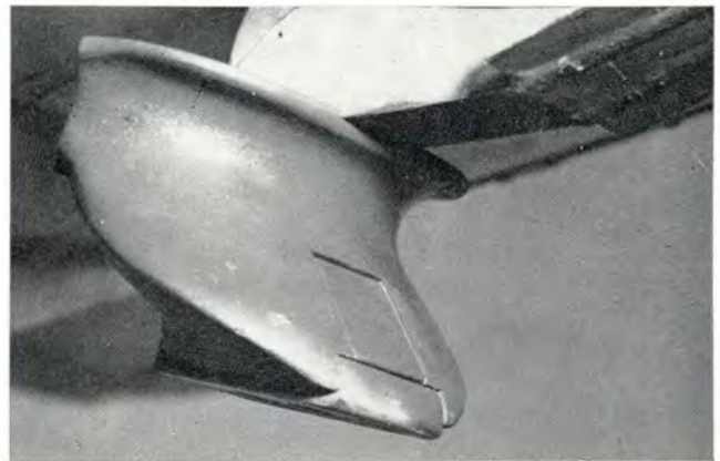
Below. Deployment reliability is insured by use of simple release mechanism. Pilot deploys the hook with a single-pull toggle switch.
