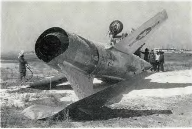
Above and right. This F-104 was using a barrier for its arrestment. Only one of the main gears caught the arresting cable and it flipped over. The pilot had no canopy, so he crawled out without trouble.
