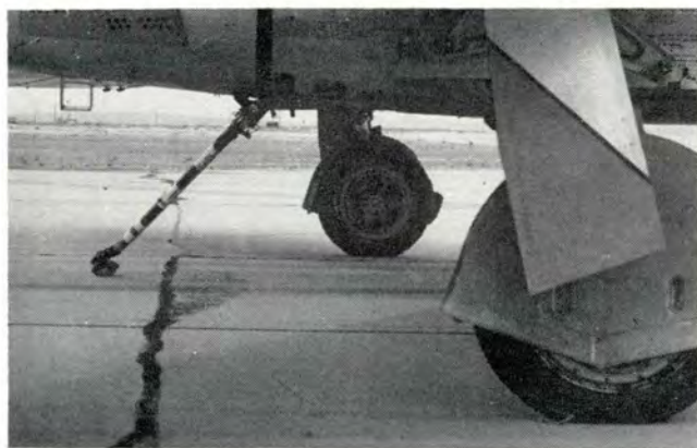
Above. The F-84 installation shows a hydraulically operated hook. Below. If arrestor cable is installed permanently above ground, tire casing supports can be used to keep cable 3 1/2-6 inches off runway.
